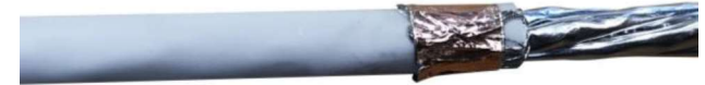
3. paste copper foil on the braid and ground wire and cut off the excess weave and ground wire
