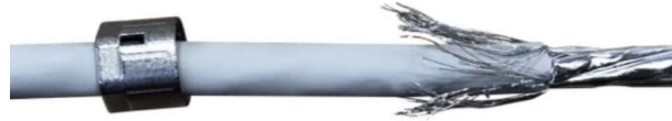
2. strip off 1.2 inch(30mm) of cable jacket, fold back braid and drain wire.
